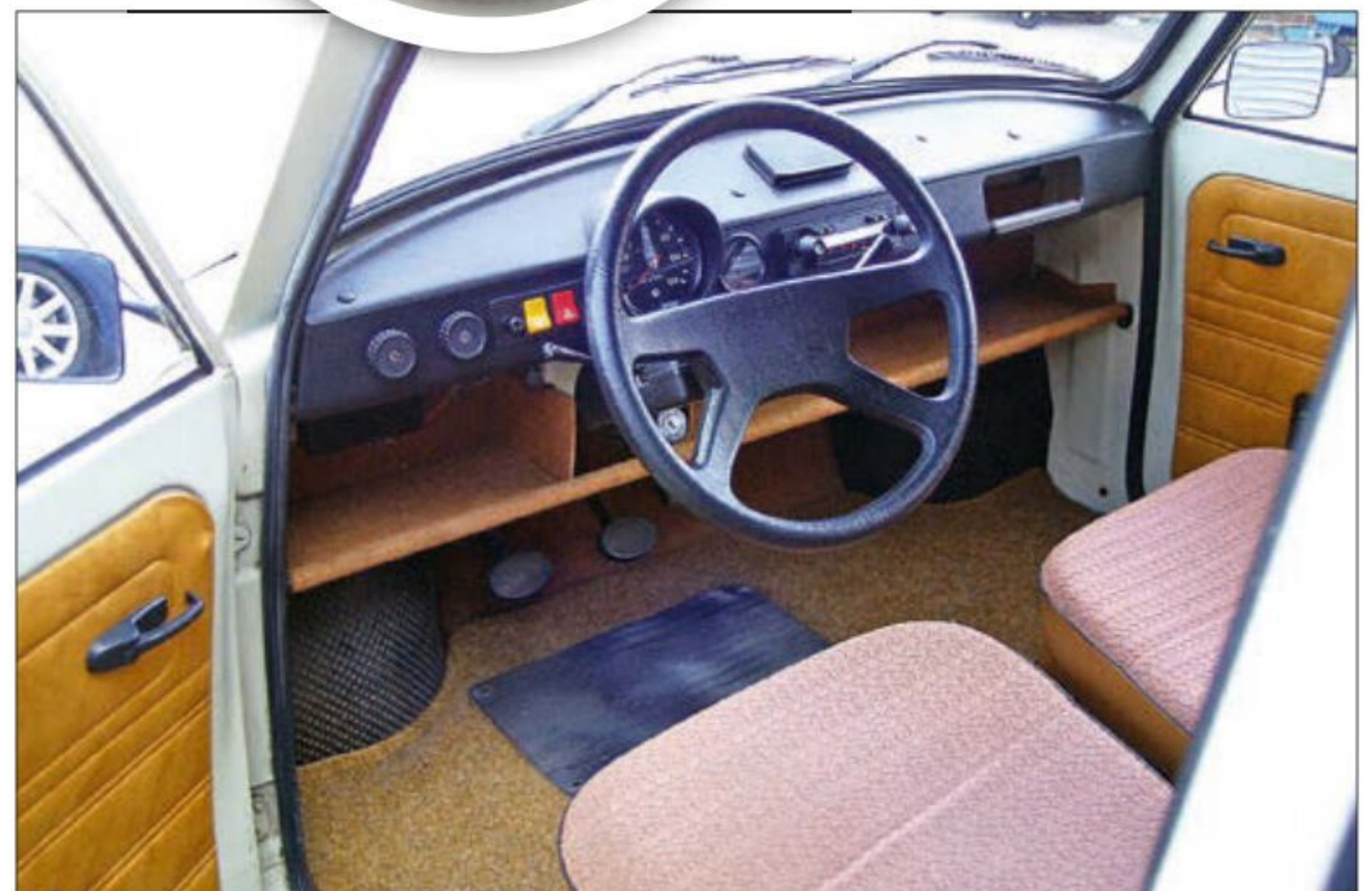
A column gear change on the two-stroke cars (four-stroke versions got a floor-mounted stick) and a flat floor from the FWD layout.
