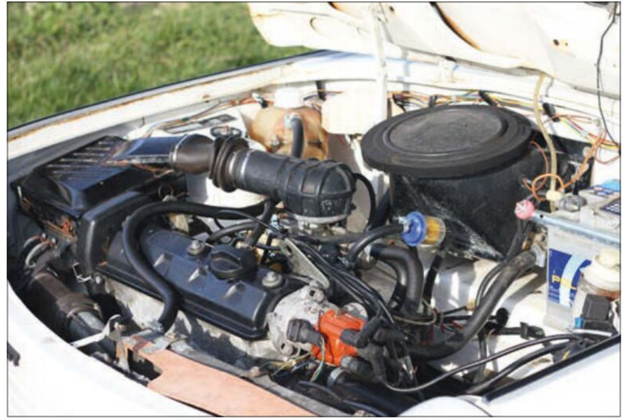
Most Trabants had a two-cylinder, air-cooled, two-stroke engine (left), but a few got a 1043cc four-stroke unit from the VW Polo (right).
