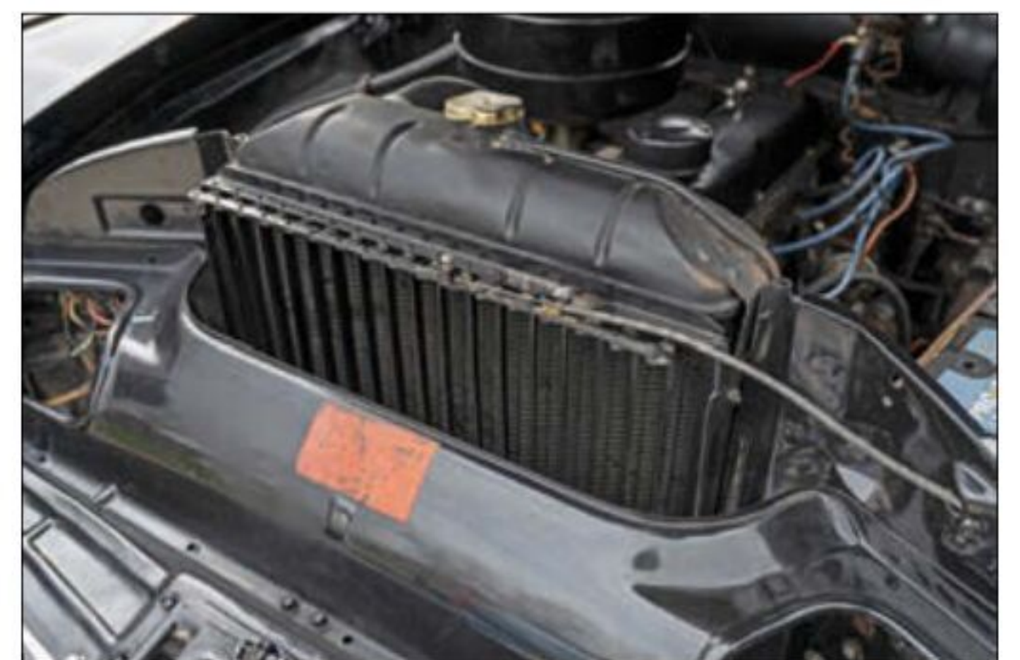
The radiator blind is connected by a cable to a lever on the dashboard.
