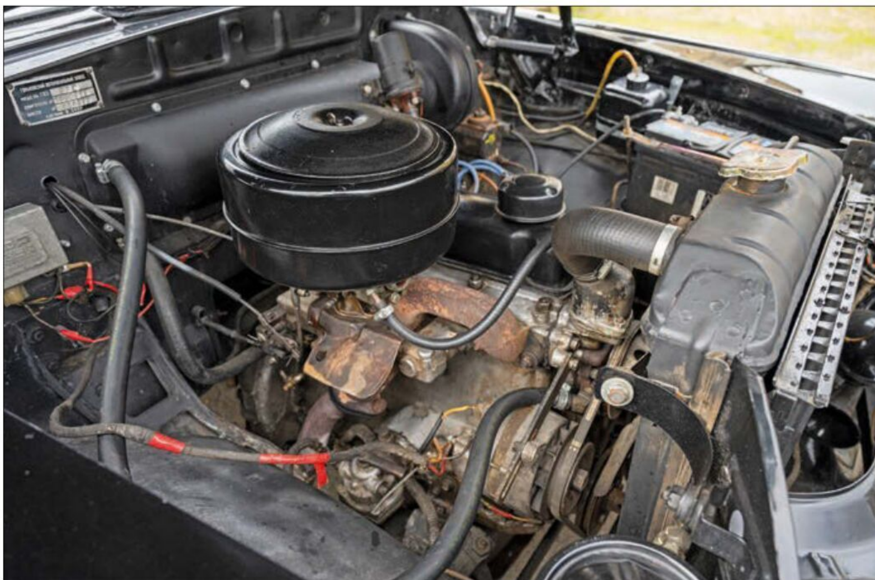
Everything about this car is over-engineered, including a 2.4-litre alloy OHV four-cylinder engine.
